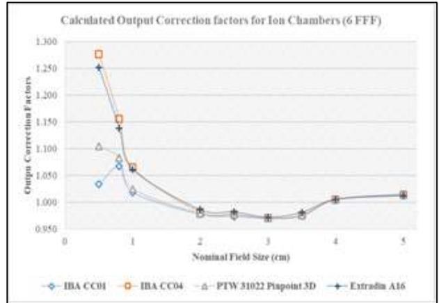
Figure 5c: Ion chambers output correction factors at 10 cm depth for 6FFF.
