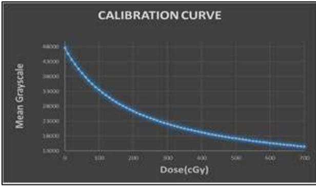
Figure 4: Calibration Curve for 6WFF Photon beams
