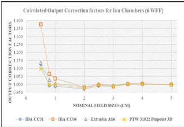
Figure 5a: Ion chambers output correction factors at 10 cm depth for 6 WFF.
