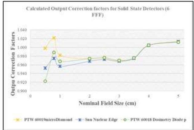
Figure 5d: Solid-state detectors output correction factors at 10 cm depth for 6FFF.
