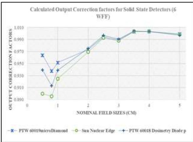
Figure 5b: Solid-state detectors output correction factors at 10 cm depth for 6WFF.
