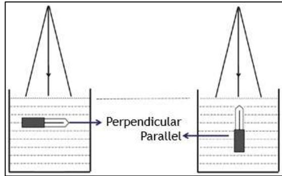
Figure 2: Detector orientation inside water phantom.
